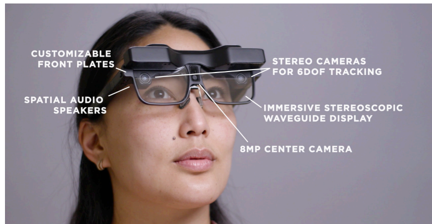
Modular and flexible head worn platform using the Qualcomm® Snapdragon™ XR2 Platform
