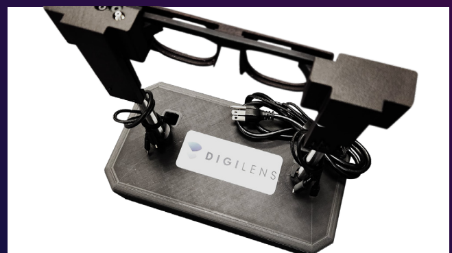
Top view of display system showing slots for swappable waveguides and left side binocular alignment screws
